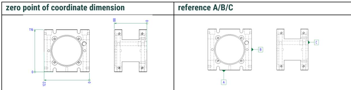
For undimensioned elements, the following always applies: The dimension from the zero point is assigned the corresponding tolerance (general tolerance or tolerance assigned via colour).
