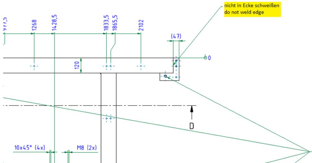
All non-tolerated dimensions and unmachined surfaces of welded parts shall be manufactured in accordance with the general tolerance DIN EN ISO 13920 B.
