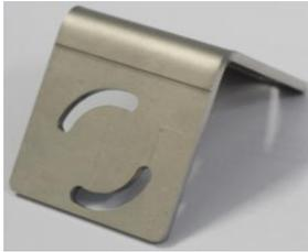
Impression caused by the bending.
